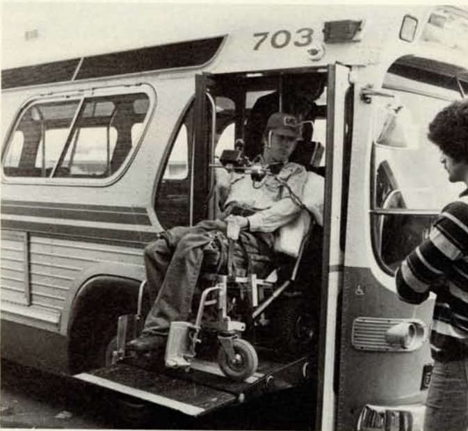
TESTING LIFT — Young Concord resident takes test ride on prototype wheelchair lift. Developed by Environmental Equipment Corp. of San Leandro, device was installed for evaluation in special demonstration service begun in Concord as part of AC Transit's continuing effort to provide wheelchair accessibility.
