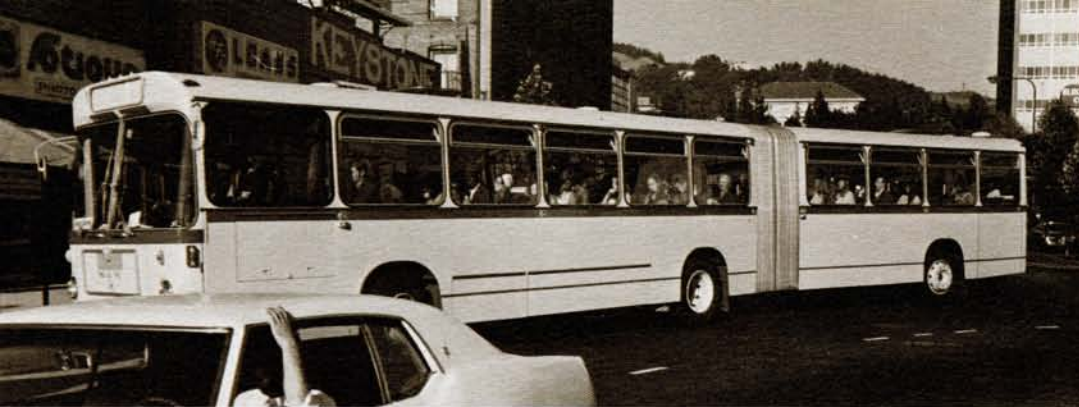
One of two European made articulated buses tested by AC Transit bends around a corner in Berkeley, as passengers enjoy the ride in a bus 54 feet long that seats 62 passengers. Surveys taken during testing showed positive rider reaction to the double buses. Specifications now are under preparation and the District may be going out to bid for the buses in the coming year.
