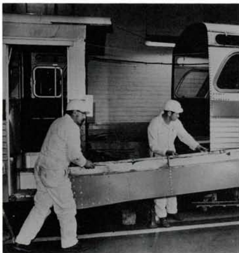
Maintenance workers remove a six-foot section from standard size bus, one of 13 converted for use in Dial-A-Ride. The bus was cut from 35 feet long to 29 feet.
