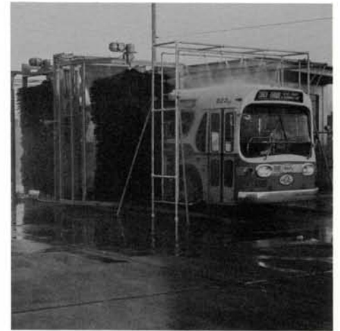
Equipment acquisitions during the past fiscal year included this bus washer installed at the Richmond Division. The machine houses nine-foot nylon brushes which can clean a bus exterior during a 63-second pass-through.
