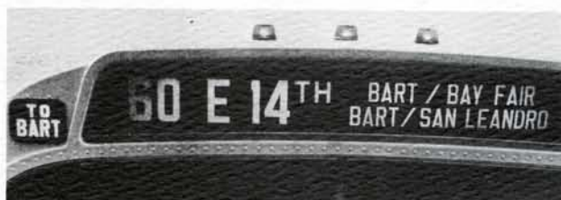
Special "To BART" light and new headsign insert informs waiting passengers this bus is headed to a BART station.
