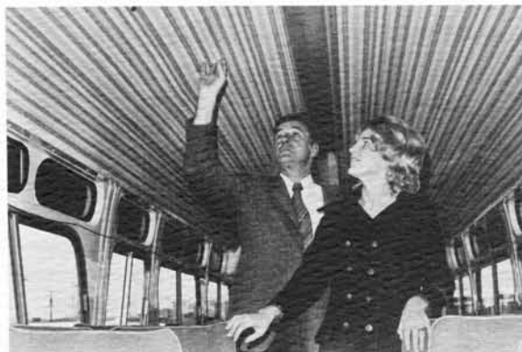
Carpeting on the ceiling? There's a reason for it. The carpeting, installed on one of the transbay buses, is part of an experiment to reduce interior noise. Maintenance Manager A. R. Lucchesi and PBX/Information Clerk Kathy Fischer examine installation.
