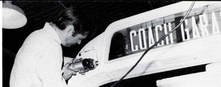
Darell Willis, Emeryville maintenance worker, cuts space for new "TO BART" light which will inform waiting passengers that an oncoming bus is going to a BART station.
