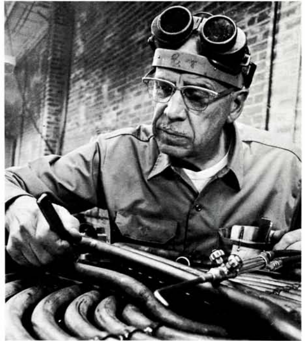
Barney Becker, who has spent 45 years in steam, welds away at 1400 feet of steel tubing which will go into the steam generator.
