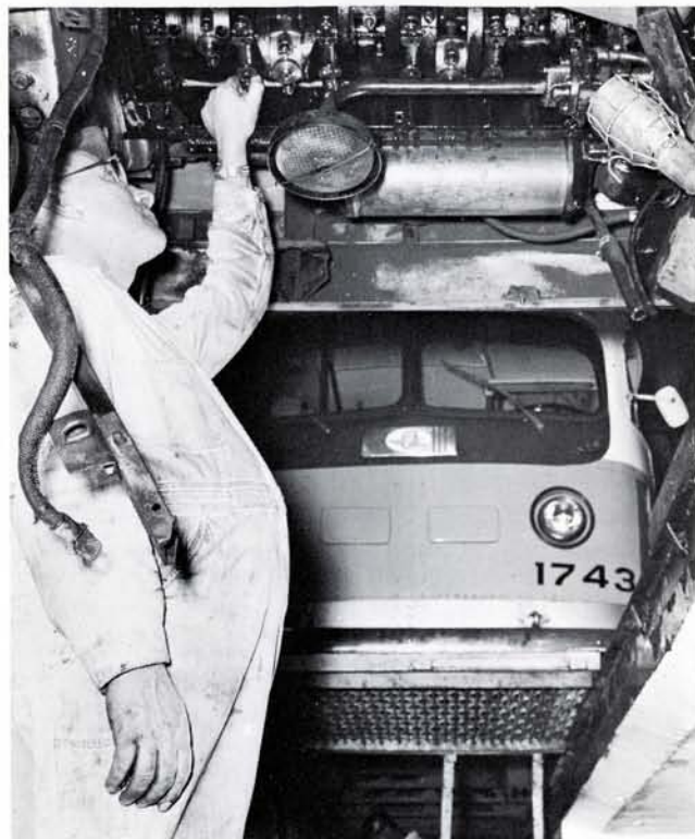
Standing in maintenance shop pit, mechanic inspects diesel engine of AC Transit bus as part of regular 200,000-mile overhaul.
