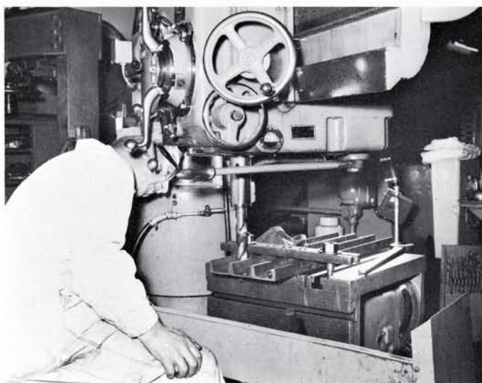
Large drill press bores through pieces of metal to be used in replacing worn or damaged sections on bus chassis.
