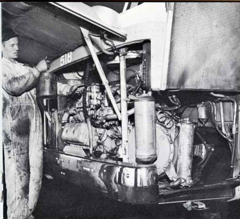
Mechanic changes oil filter in diesel engine at rear of bus as part of 5,000-mile preventative maintenance check-up.
